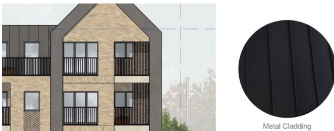
Figure 14: rolled joint metal cladding
