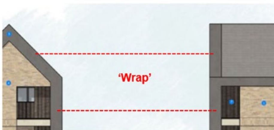
Figure 8: metal clad gable and wrap to side elevations and metal verge detail
